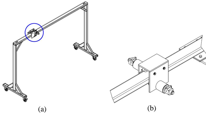
Figure 2: (a) Gantry crane structure; (b) Magnified trolley section
