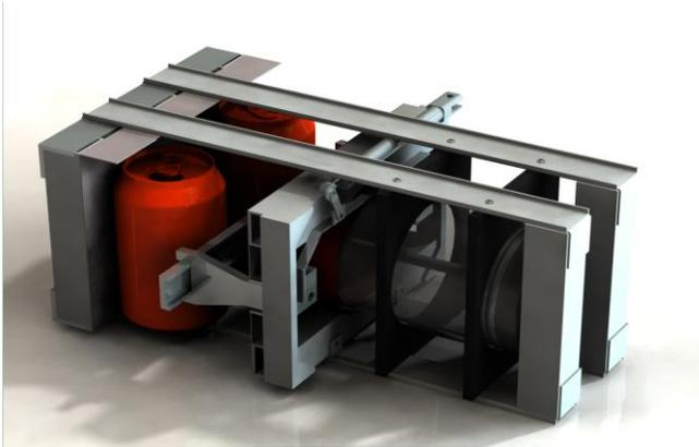
**Figure 4. An example of a student’s solid model – Julie Henion’s can crusher.**
