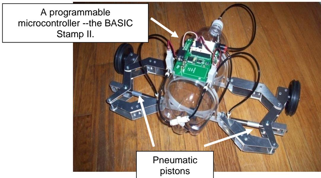
**Figure 1. The compressed air powered robot built in 2.670 in IAP of 2009.**
