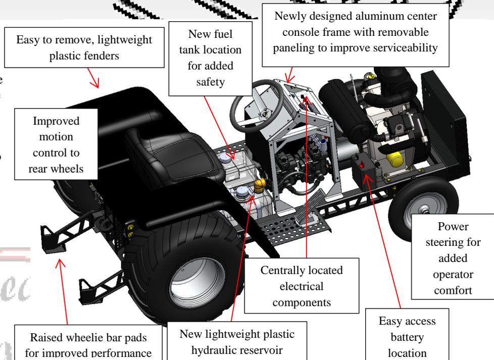
**Figure 5:** SolidWorks model of 2014 EHPP showcasing design improvements (with some ABS plastic paneling removed). One can notice the relocation of the fuel tank to a location inside the frame rails along with relocation of the battery to provide easy access for installation, removal, and external charging.
