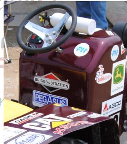
**Figure 4:** Picture showing poor control labeling and layout along with lack of instrumentation on 2011 EHPP.
