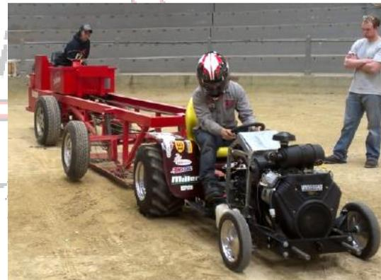
**Figure 2:** Test pulling at UW-Madison's testing facilities on April 12, 2014, to test the initial iteration of control programming and redesigned operator interface and control/instrumentation layout.
