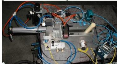
Figure 1, PID position control setup
