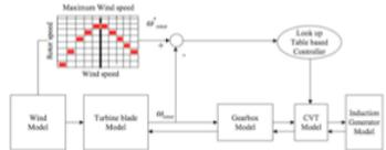
Figure 2 Block diagram of the simulated wind power turbine drivetrain
