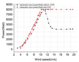
Figure 3 Simulated comparison between a fixed ratio and variable ratio wind power drivetrain
